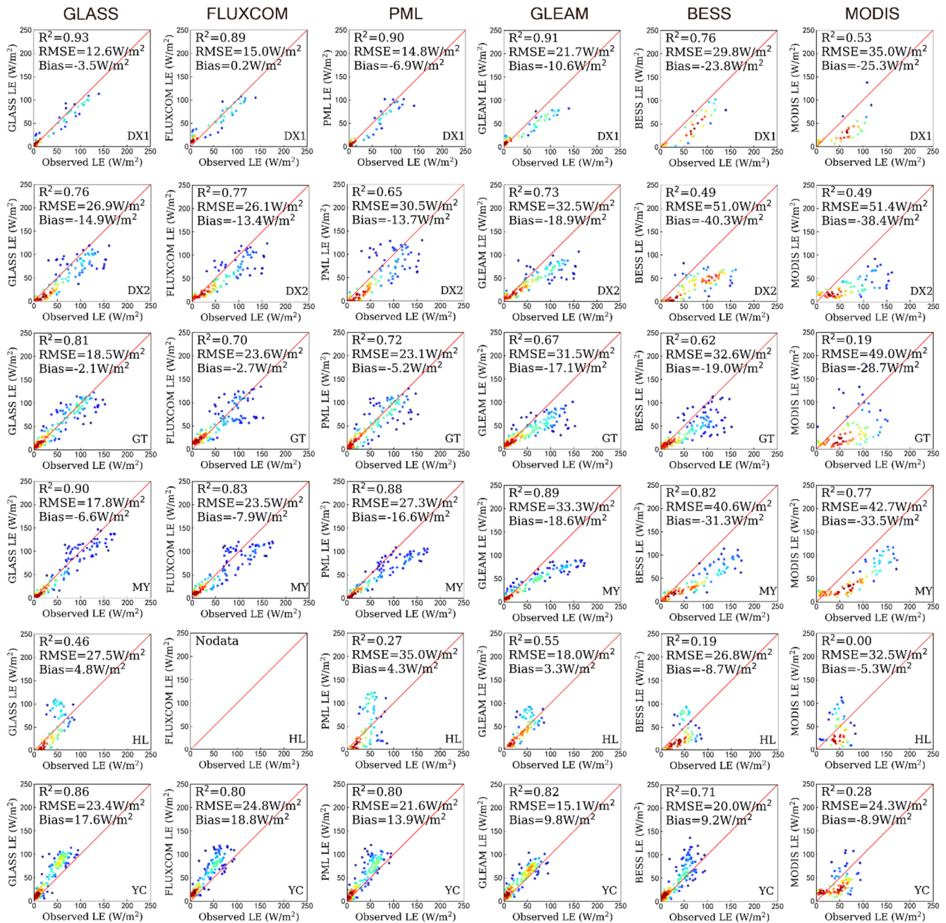
Figure 2. Scatterplots of the observed LE and estimated LE derived from six LE products at six different sites.
