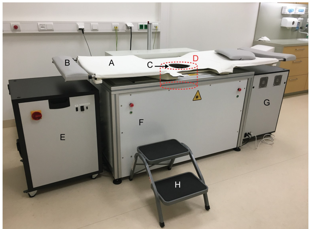
Fig 1. PAM 2 system in hospital setting with (A) the bed on which a woman lies prone, (B) a foot rest, and (C) the breast aperture with (D) a schematic of the shape and position of the imaging tank below the bed, (E) the power supply and cooling unit, (F) laser head (behind the panel), (G) DAQ unit, and (h) step stool. Reproduced from Ref. [11] with permission of authors and publisher.
