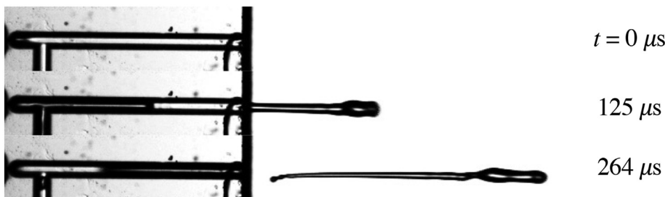
FIG. 4. The jetting sequence of a fully filled CA1 channel. The panels show the moments of jet emergence from the channel (top), maximum bubble size (middle), and complete bubble collapse. Multimedia view: https://doi.org/10.1063/5.0143223.1
