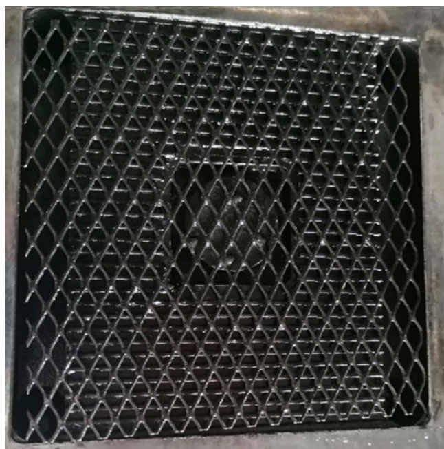
Figure 1. Flow geometry of the electrode compartment: Pt/Ti mesh on top, perpendicular flow field below, a manifold both for the inlet and for the outlet, all contained in plastic housing. The dark color of the electrode originates from its use with the carbon-based slurry electrode.
