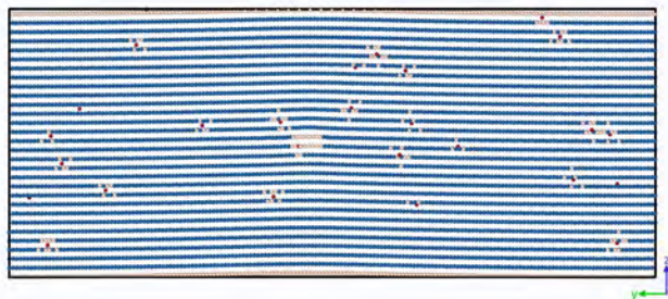
Figure 2: \{110\}\langle 111\rangle edge dislocation setup in iron. The blue atoms denote the bcc symmetry of the Fe atoms, while the red atoms between planes resemble the H atoms.
