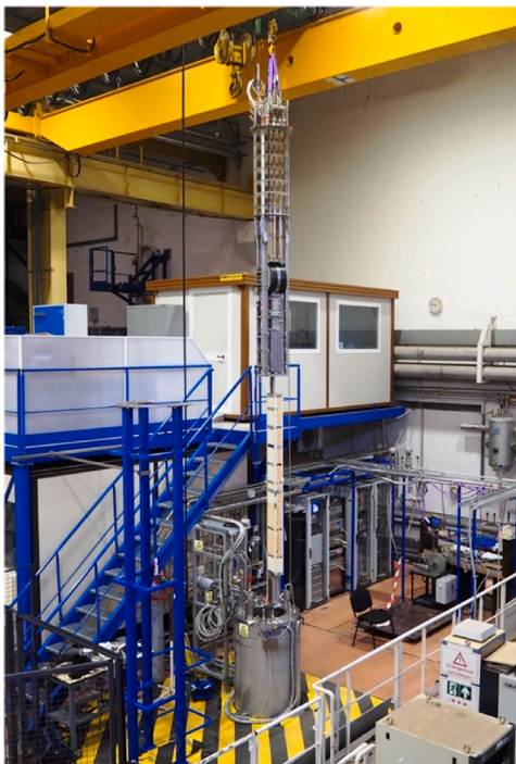
Fig. 10. Test assembly insertion inside the cryostat.
