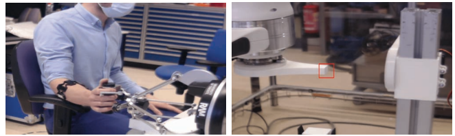
Fig. 3. Setup of the user experiments. Left: user operating Omega 7 leader and wearing Myo EMG sensor. Right: user view of the robot end effector (left side of image), with alignment square, facing the contact target (right side of image).
