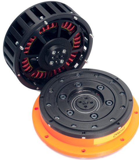
Fig. 1: Cycloidal drive prototype with motor and gearbox separated.
