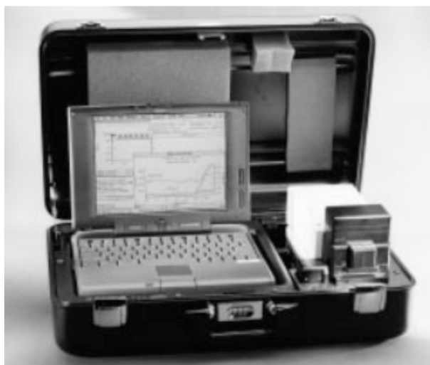
Figure 1. A photograph of the MATCI, which was the size of a briefcase and was rechargeable battery-operated. Reprinted (adapted) with permission from [13]. Copyright 1998 American Chemical Society.
