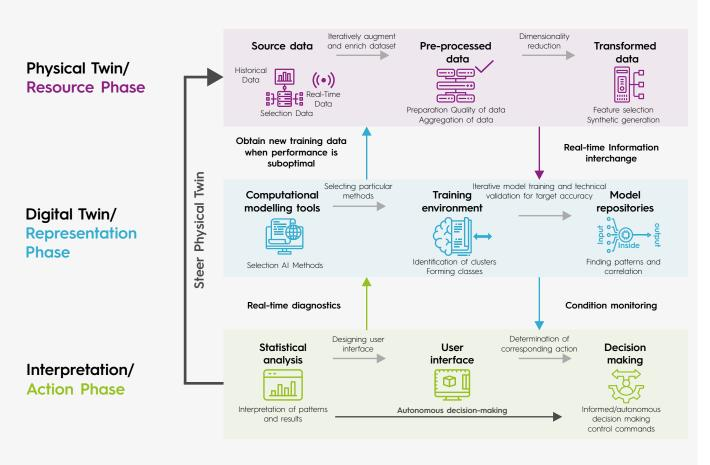
Figure 1. Conceptual diagram covering the whole Digital Twin development cycle
