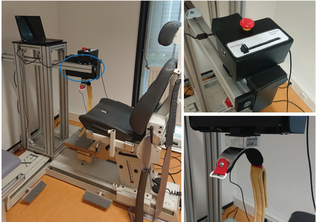
Figure 7.1 | Photos of the setup. The close-up on the top right shows the comfort slider with VAS and the close-up on the bottom right shows the thigh cuff with straps. The actuator unit is located inside the black cover between the comfort slider and the cuff (circled in blue).
