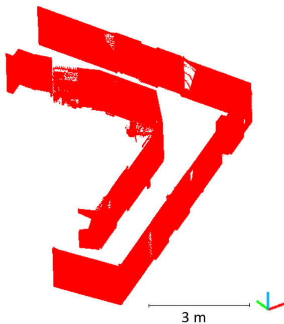
Figure 5. Slanted view of the TLS 3D point cloud for the ITC1 dataset. The ceiling and floor points are not shown for visualization purposes.
