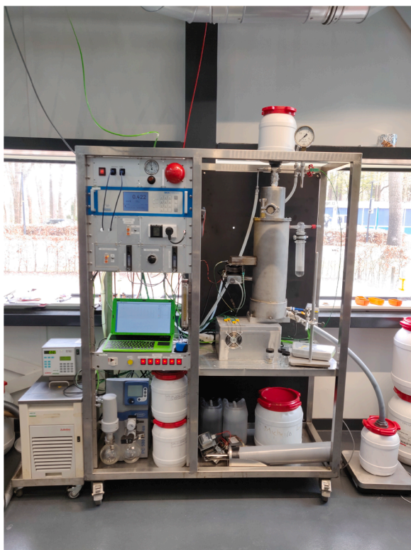
Fig. 5. Picture of the microwave desorber setup.
