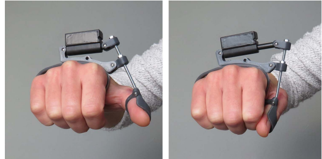
Fig. 1: Overview of the T-GRIP thumb exoskeleton that supports the lateral pinch grip. The force transmission mechanism is shown with the thumb in extended (left) and flexed (right) position.
