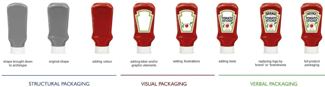
Fig. 1 Heinz Ketchup bottle build up from structural, to visual, to verbal packaging cues
