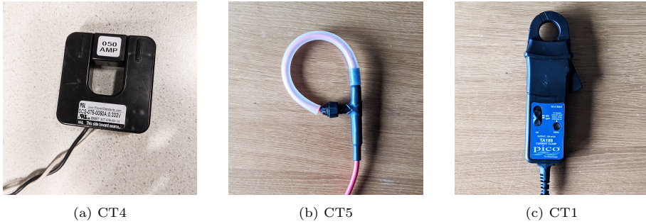
Figure 4.10. Photograph of the used CTs.
