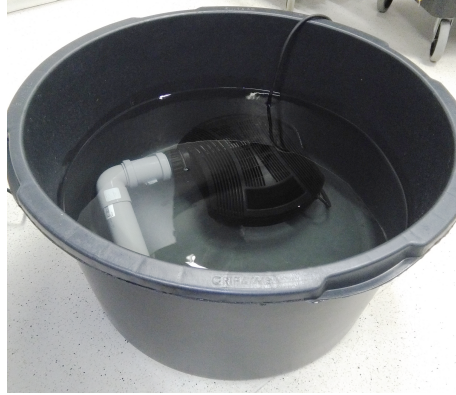
Figure 3.4. Picture of the COTS water pump placed inside a circular container filled with water.
