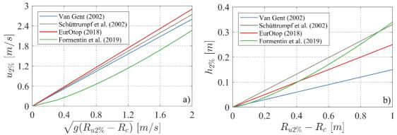
**Figure 1.** Comparison of existing empirical equations for a) overtopping flow velocity and b) layer thickness at smooth slopes; A slope of 1/4 was applied for calculations using EurOtop (2018) equations and Formentin et al. (2019) equations.
