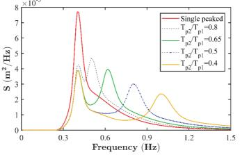
(a) Wave energy spectra with the lowest peak frequency at  $T_{p1} = 2.5$  s.
