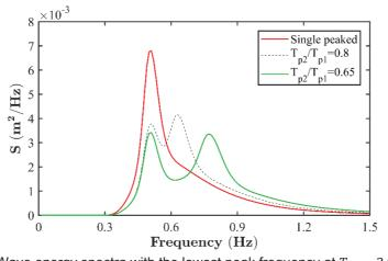
(b) Wave energy spectra with the lowest peak frequency at  $T_{p1} = 2.0$  s. **Figure 3.** Single and double-peaked wave energy spectra based on which the irregular waves were generated according to Van Gent (2002b).
