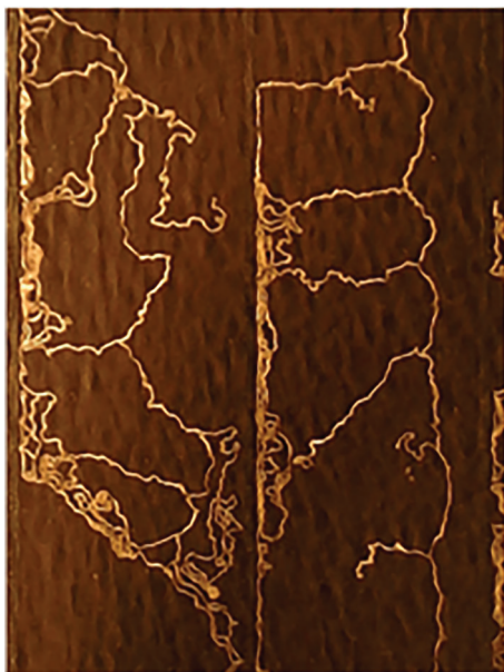
FIGURE 8 A close-up image of wormlike defects in two interconnected cells of a CIGS module exposed to partial shading stress. 88
