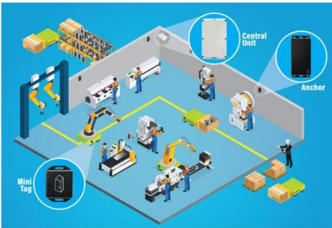
Fig. 3. Illustration of an RTLS set-up showing tags and anchors for collecting real-time data from tags [17].
