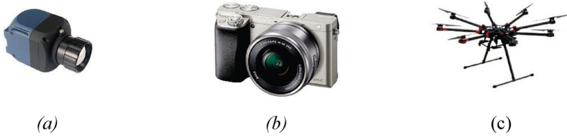
Figure 4. Thermal camera (a) RGB camera (b) and UAV platform (c) used in study.
