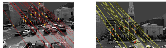
Figure 8. The image point correspondences and the epipolar lines on the stereo images using photogrammetric coplanarity or collinearity equations.
