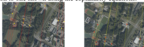
Figure 17. The image point correspondences and the associated epipolar lines on the stereo images using the fundamental matrix in test 2.
