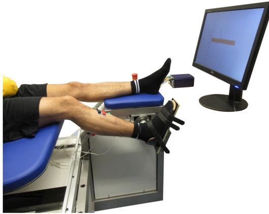
**Figure 6.1: Experimental Setup.** Participants were seated on an adjustable chair for the instrumented evaluations. The manipulator connected to the adjustable chair applied dorsiflexion, ramp-and-hold perturbations around the ankle joint, while measuring the biomechanical response. If the left foot was measured, the right leg was supported with a right lower leg support inserted into the chair frame (not shown).
