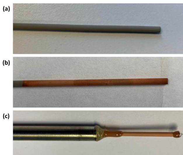
Figure S4.1. Photograph of (a) Ti hollow fiber, (b) Cu-Ti hollow fiber and (c) Cu-Ti electrode assembly.
