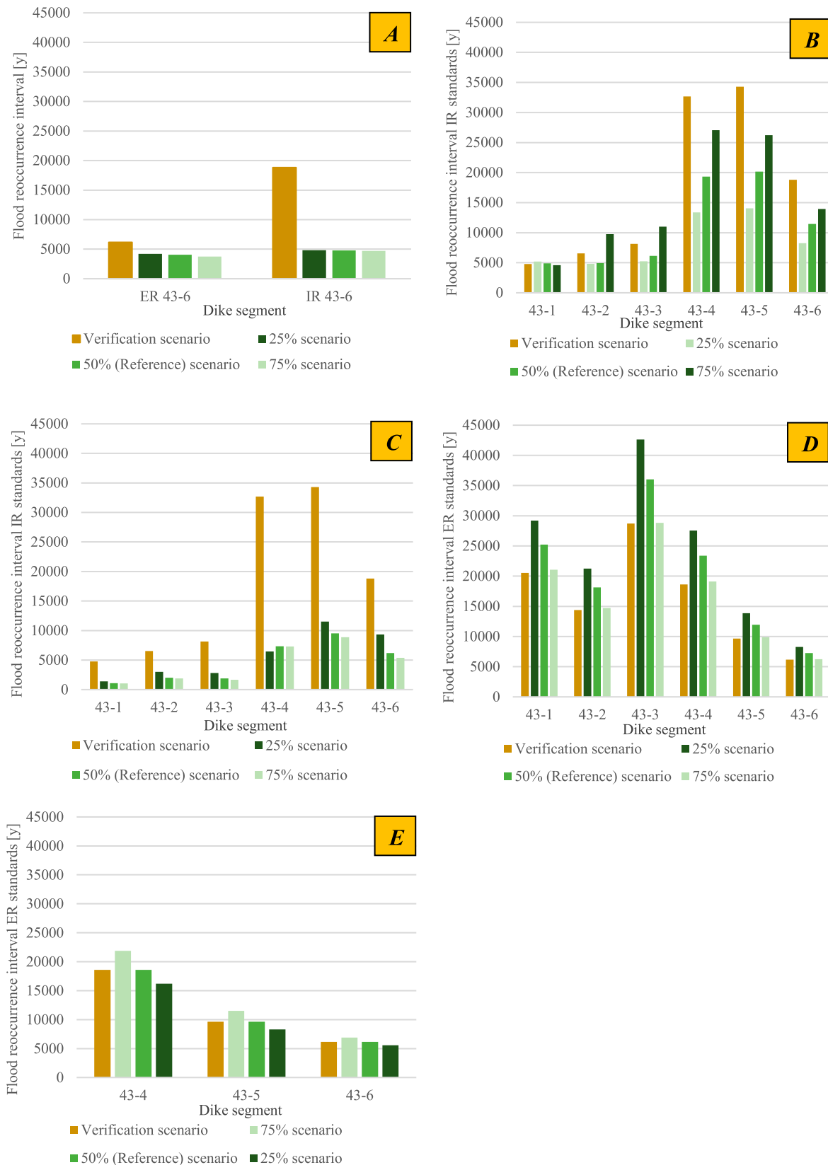
Figure 5. Influence of scenarios per uncertainty source on the flood safety standards for the individual dike segments. (A) Breach development; (B) Mortality functions; (C) Evacuation; (D) Damage functions; (E) Flood defence investment costs. Note: A shows the influence for both IR and ER standards, B and C show the influence on IR standards and D and E show the influence on ER standards.
