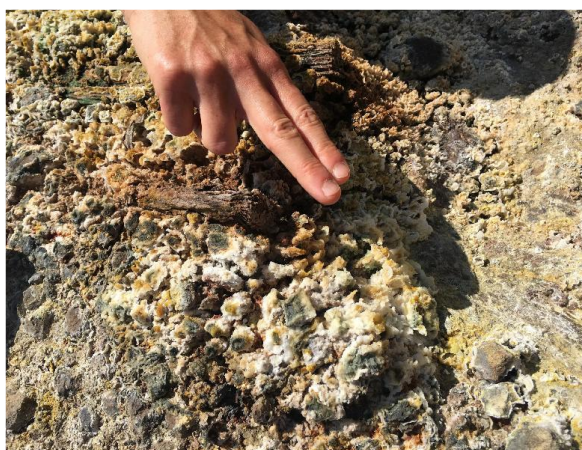
Figure 3 - Silica sinters (sample MATA2) deposited adjacent to the Mataloko geothermal plant on Flores Island which is ongoing precipitating and evidences the modern fluid activity in the field.
