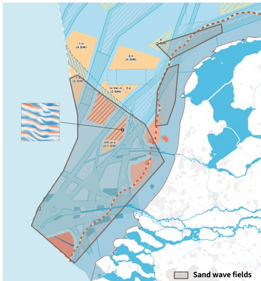
Figure 1.1: Planned and constructed offshore wind farms in the Southern Dutch North Sea (indicated by the coloured areas). Shaded regions indicate approximate locations of sand waves (areas retrieved from Németh (2003), figure adapted from RVO, Rijksoverheid (2022))
