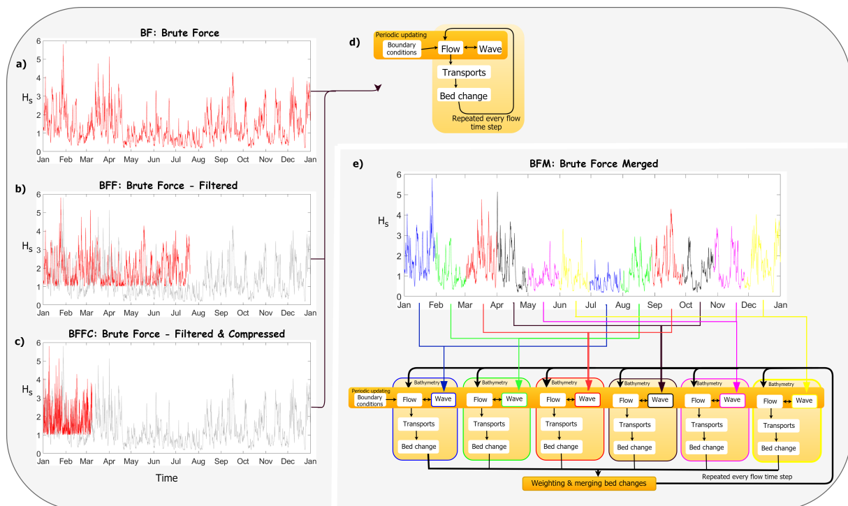
Figure 4.2: Schematization of acceleration methods used in Luijendijk et al. (2019) to reduce computation times of a flow model including waves: a) Brute Force (BF), no acceleration, b) Brute Force - Filtered, using input filtering, c) Brute Force - Filtered and Compressed (BFFC), using input filtering and time compression (combined with MF) and e) Brute Force Merged, using compression (combined with MF) and parallelization of wave conditions. d shows the morphological feedback loop in the BF, BFF and BFFC cases.
