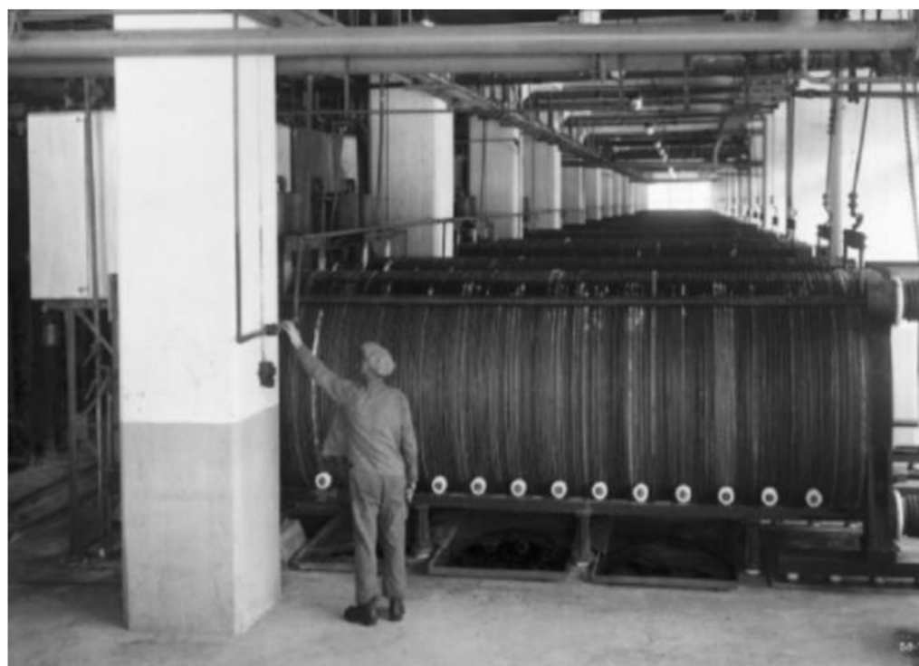
Figure 7. Electrolyzers at the Rjukan ammonia factory in Norway, operational 1928–1971. Courtesy Norsk Hydro.
