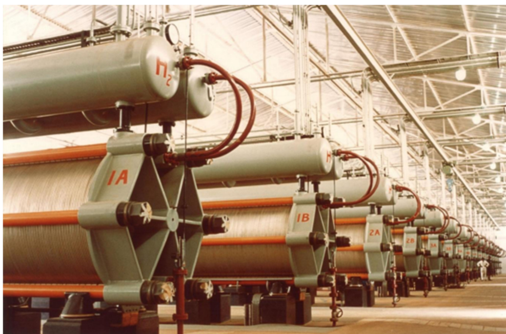
Figure 9. Top: Electrolyzers at the Cuzco ammonia production facility. Reproduced from reference [43]. Bottom: Electrolyzers at the Kwekwe ammonia production facility. Reproduced from reference [43].
