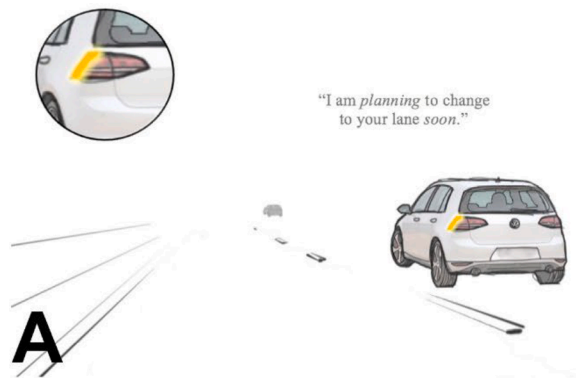
Fig. 1. Illustration of the enhanced semantics visualized in a turn signal.
