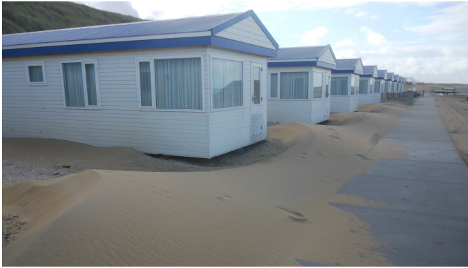
Figure 1.3: Deposition in front of a row of holiday houses at the beach (Katwijk, The Netherlands)
