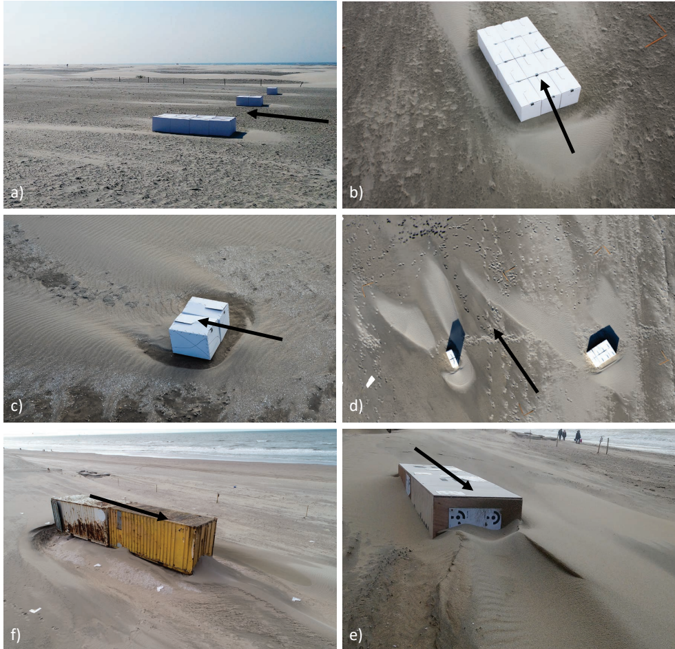
Figure 3.12: Examples of deposition around scale models, with arrows indicating the (dominant) wind direction. a) Small scale models of different length, with upwind deposition and deposition tails visible as lighter areas (29-05-2018). b) The nearest small scale model of photo a from another angle. c) Deposition with a considerable elevation difference (23-10-2018). d) An orthophoto of deposition (12-10-2018). e) The full-scale model of the 5-week experiment, showing deposition, erosion and undercutting under the upwind side of the container (11-03-2020). f) The small scale model of the 5-week experiment, half-buried and with a deposition tail downwind of the model (11-02-2020).
