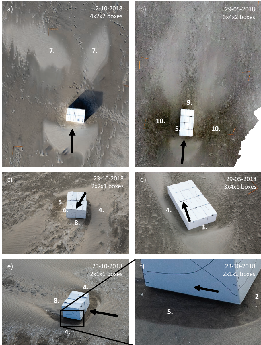
Figure 2.6: Notable erosion and sedimentation structures around scale models, with arrows indicating the wind direction. a) Orthophoto showing a large distance between the model and the start of the downwind horseshoe deposition. b) Orthophoto showing lateral inner and outer erosion and downwind inner erosion. c) Photo of a model oriented obliquely to the wind, showing lateral inner deposition d) Photo of model a oriented obliquely to the wind, showing upwind inner deposition and asymmetric lateral deposition. e) Photo showing continuous lateral deposition. f) Zoom of 6e, showing erosion around model and under model corners.
