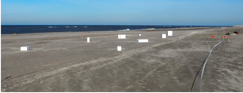
Figure 2.2: A photo of one of the set-ups, testing the effect of building width and height (12-10-2018)
