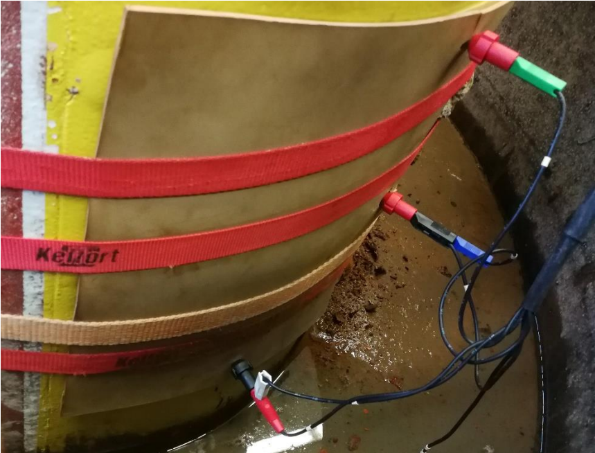
Figure 34. Image of the CA I prototype on the mono-pylon to test sea water immersion exposed part of a heavy-duty maritime coating. The sensor was fitted with stripes and thick leader laminate on back plate of the sensor.
