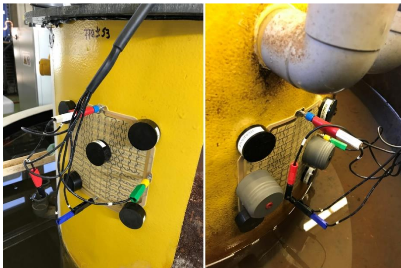
Figure 39. Application of generation II type concentric array sensor for characterization of coating applied on model offshore pylon above (left) and below water line (right). The sensor
