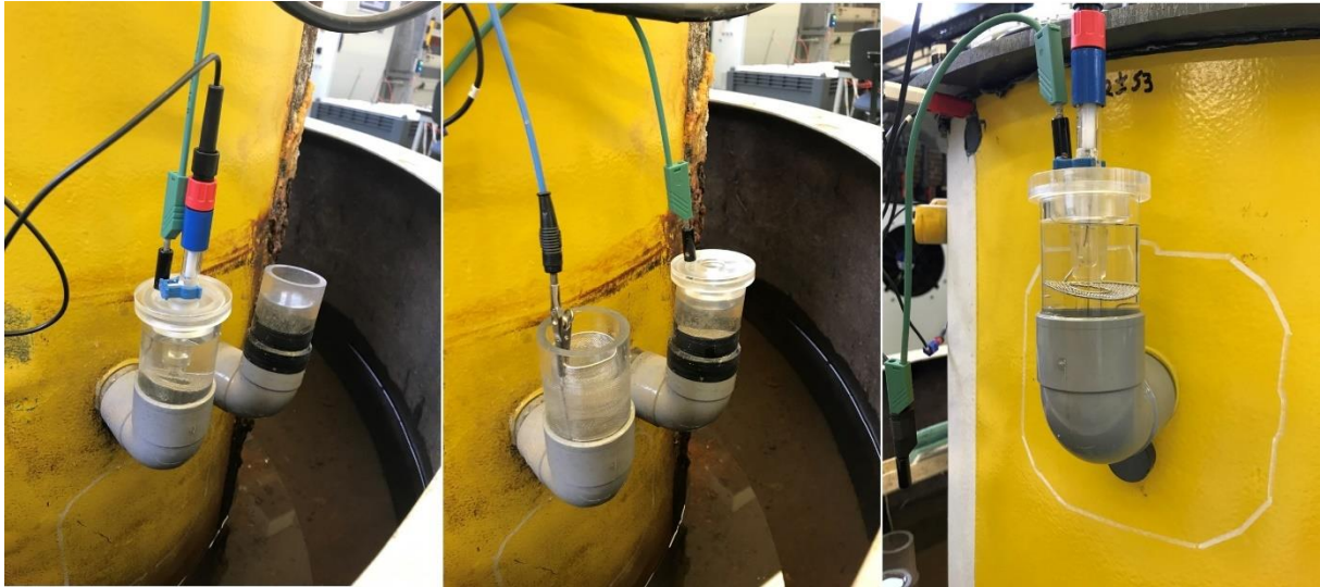
Figure 38. Application of traditional wet phase test setup for characterization of coating applied on model offshore pylon above and below water line. The one cell setup with direct wire connection to the substrate (left) and the two cells setup without direct wire connection to substrate (middle) located on coating surface below water line, one cell setup with direct wire connection to substrate above water line (right).
