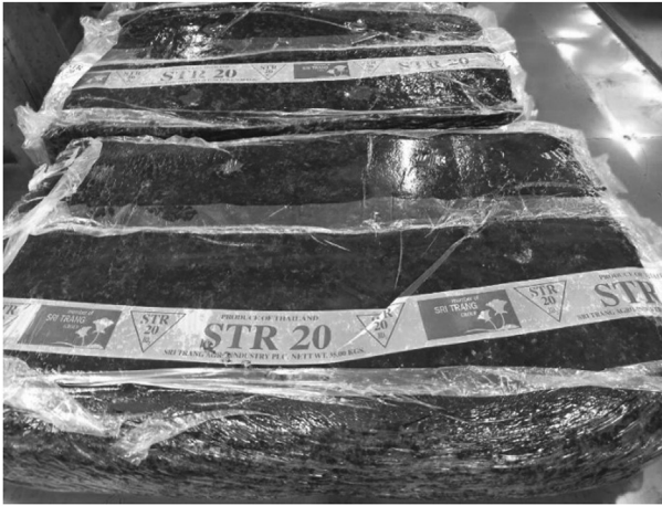
Figure 9.2 STR20—one of the TSR, as the most commonly used raw NR for tire productions. STR20 , Standard Thai Rubber grade 20; TSR , technically specified rubber.
