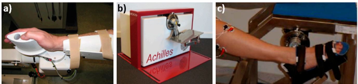
Figure 3. Wristalyzer robot (a), Achilles robot (b) and Achilles during use (c). Courtesy of Amsterdam UMC, TU Delft and LUMC.
