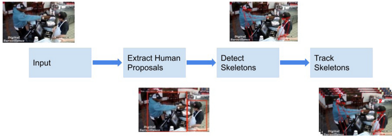
Fig. 1. Feature extraction pipeline of HR-Crime dataset. Given the frames of a video, we first extract human proposals using YOLOv3-spp [5]. Second, AlphaPose [3] is applied to detect body skeletons. Finally, PoseFlow [17] is used to track skeletons.
