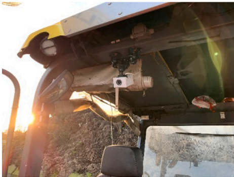
(c) IR camera on the paver
