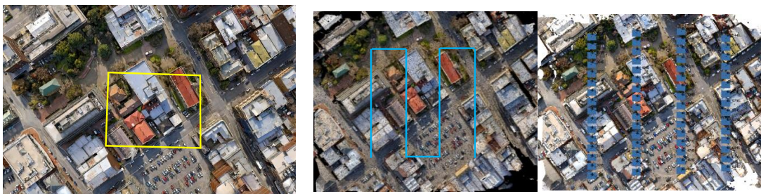
Figure 6. The Launceston 3D city model shows the area of interest inside the yellow boundary (left) and the grid flight trajectory (right).
