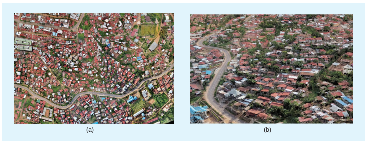
FIGURE 6. A UAV image acquired over an informal settlement in Kigali, Rwanda: the (a) 2D orthomosaic and (b) 3D photogrammetric point cloud. (Source: [147]; used with permission.)
