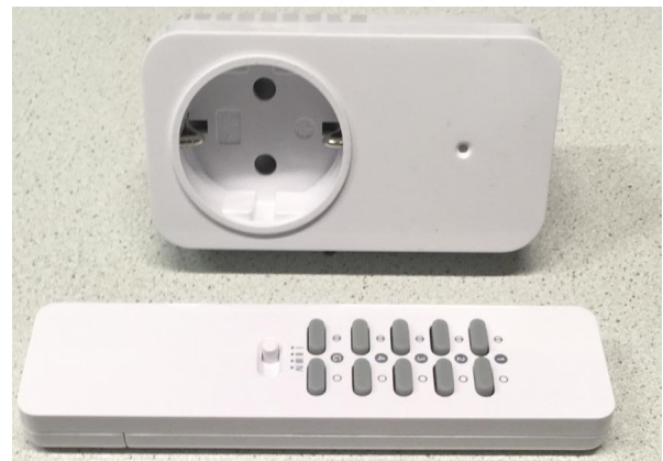
Fig. 1. COTS switch with dimming functionalities initially bought with the idea of using it as an on and off switch
