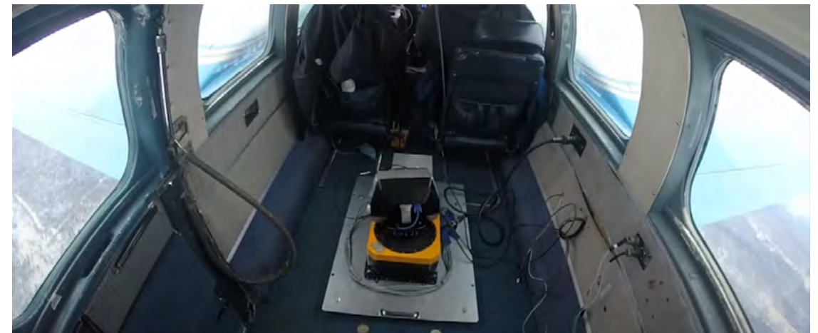
Figure 3. Hyper-Cam Airborne Mini installed in a Piper Navajo aircraft collecting data.
