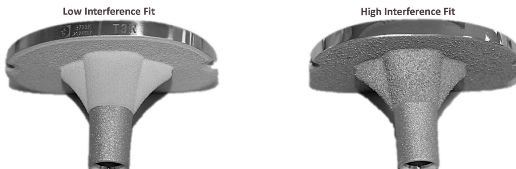
Fig. 1. Tibial components with different interference fits. Due to the adapted production method, the high interference fit implant had a higher roughness and a slightly higher dynamic coefficient of friction.
