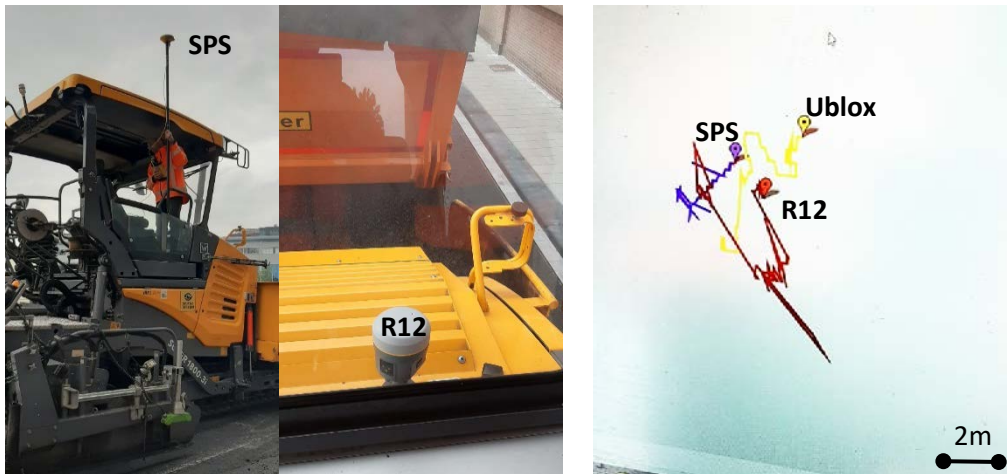
Figure 31: SPS on the roof, R12 on the hood, Ublox in the paver
