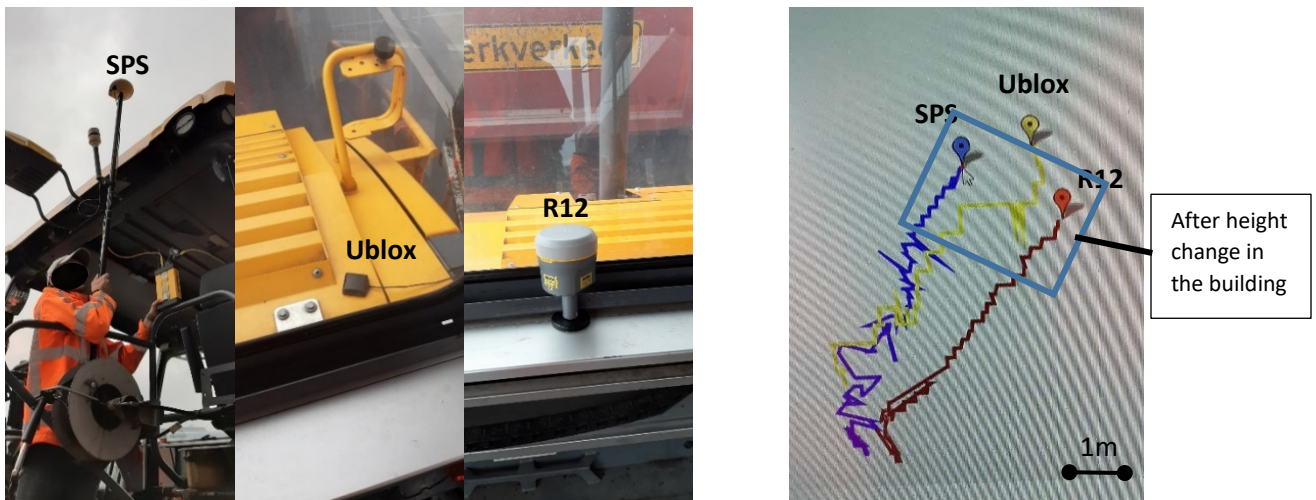
Figure 36: SPS on the roof, Ublox on the hood and R12 in the paver
