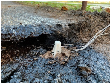
(a) placement of a 3D stand with thermocouples
