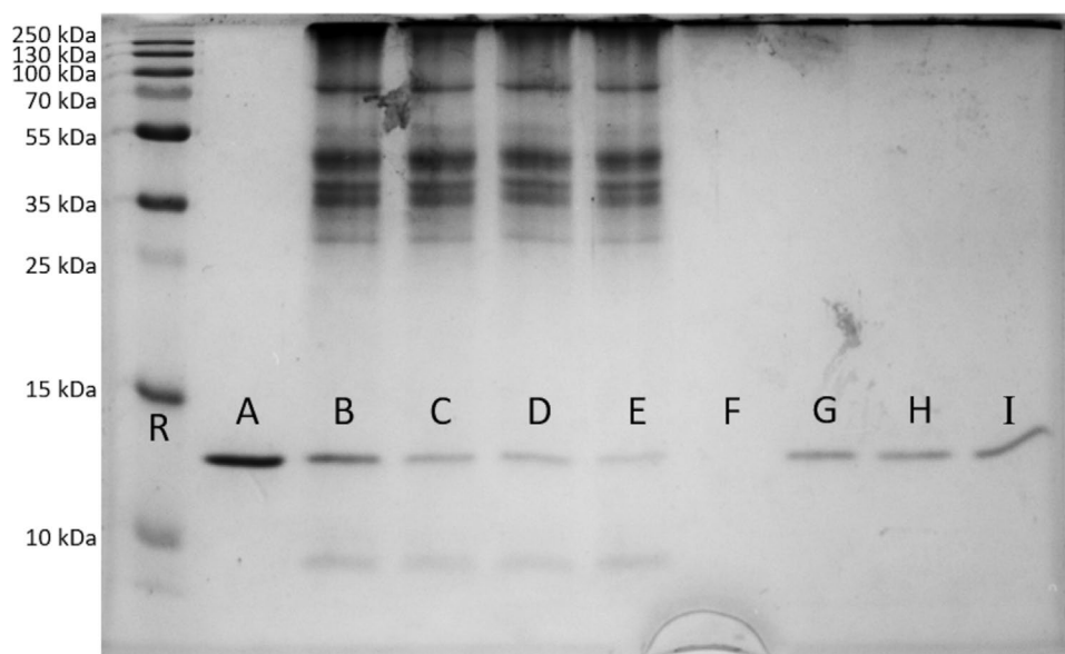
Figure 4. SDS-PAGE gels of the supernatant during extraction and release steps of 1 \text{ g L}^{-1} albumen solution. R) Reference protein mixture, A) pure lysozyme, B) 1 \text{ g L}^{-1} albumen solution, C–E) triplicate of supernatant after extraction, F) supernatant of PAH/PAA PECs without proteins, G–I) triplicate of the back-extraction supernatant after lowering the pH.
