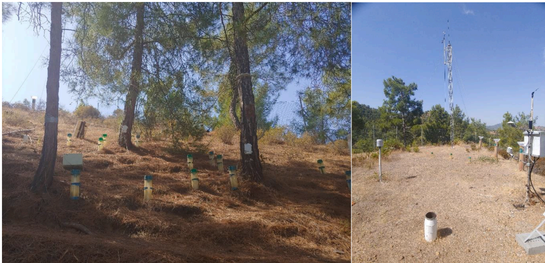
Fig. 2. Manual throughfall gauges placed around Pinus brutia trees (left) and the meteorological station at the Agia-Marina-Xyliatou forestry site (right).
