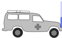
Fig. 9 A 2.4 m long vertical whip antenna mounted on a 4-wheel driven ambulance vehicle.
