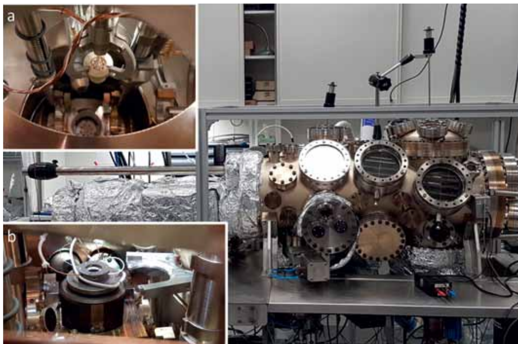
Figure 3 Ultra-high vacuum setup for in-situ scanning tunneling microscopy during deposition by e-beam evaporation (Nanolayers group). Insets (a) and (b) show views of the STM and sample holder, inside the UHV vessel. This system was developed previously at Leiden University by Vincent Fokkema and Marcel Rost.
