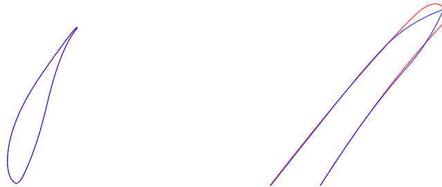
(a) Airfoil Section: Wortmann profile with Sharp Trailing Edge [129] and Actual Profile
