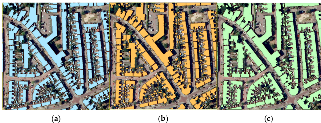
Figure 10. Results obtained on the urban area test dataset (RGB + NIR + nDSM). The predicted polygons are produced with 1 pixel for the tolerance parameter of the polygonization method. (a) Reference building footprints; (b) predicted polygons with cross-entropy and Dice as loss functions; (c) predicted polygons with Tversky as loss function.
