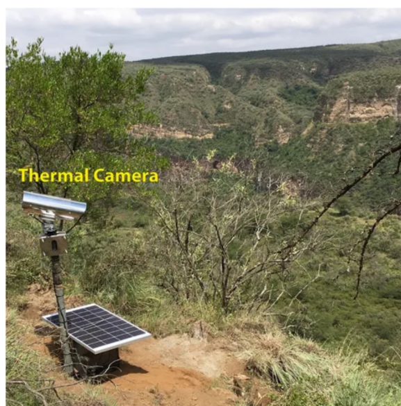
Fig. 6. The OMF6 station monitors a fumarole in the bottom of the Ol Njorowa Gorge with a thermal camera. Credit: KenGen and University of Twente
