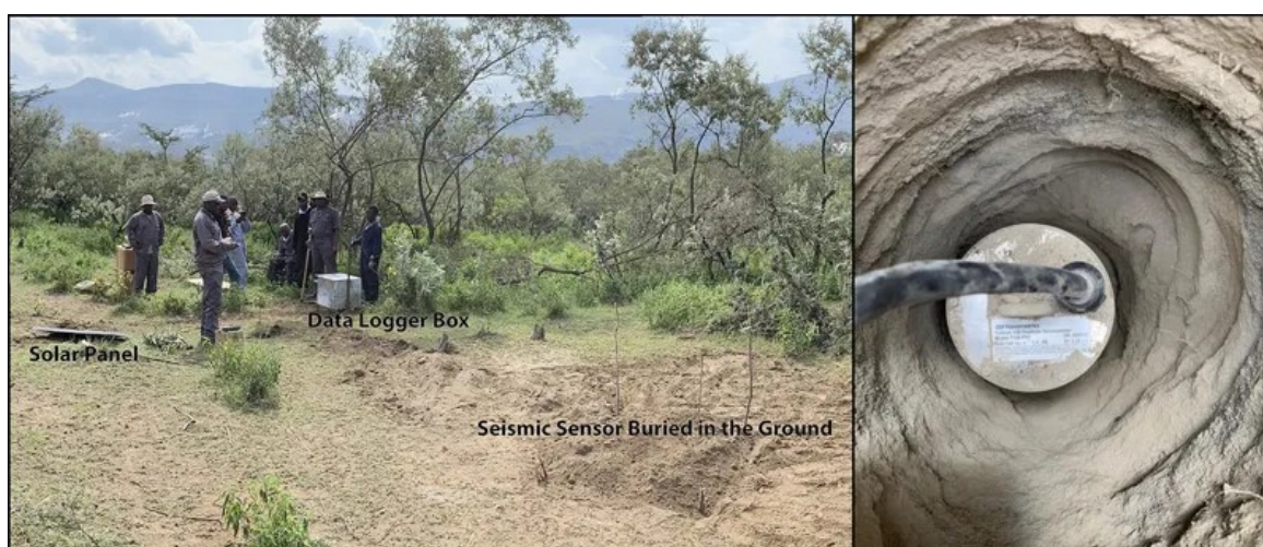
Fig. 3. Technicians stand (left) near the site of a buried posthole seismic sensor (right) in the Olkaria field lab network. Credit: KenGen and University of Twente
