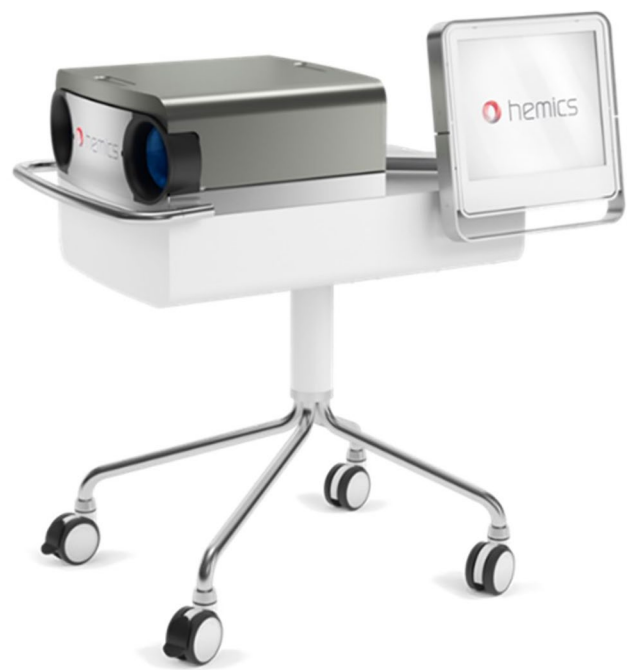
Fig. 1 HandScan. The HandScan (Demcon Hemics, The Netherlands) is a new imaging device for the detection of inflammation. Patients place both hands in the device simultaneously, resting on a plate. Red/near-infrared light illuminates the hand and the amount of light that passes through the hand is recorded by a camera. The more blood is present, the less light is passed through. The total procedure takes approximately 5–10 min and can be executed by any healthcare professional after a short training [15]. The HandScan produces a value for the level of inflammation for each separate joint and a combined score for the entire hand. The inflammation is also shown visually with a scale from green to red superimposed on the joints of the hand and wrists. This may help to understand the current activity of a patient's arthritis as well as to localize inflammatory activity. Previous research showed that the HandScan is a sensitive and specific test with good validity [15, 16]. This makes it interesting to examine the HandScan as a potential addition to or (partial) replacement of current measures for inflammatory activity such as blood tests, DAS28, MRI, and ultrasound
