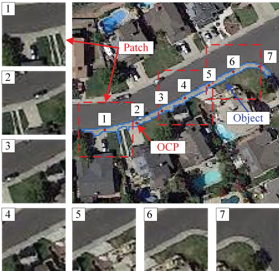
Figure 1. The concept of Object-based convolutional neural networks (OCNNs). Object convolutional positions (OCPs) (red dots) are distributed within a certain object (the blue polygon) and their corresponding patches (red dashed lines).
