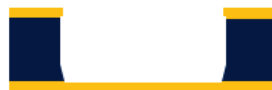
Figure 6.14. Schematic process flow for fabricating boron membranes by etching through the wafer.
